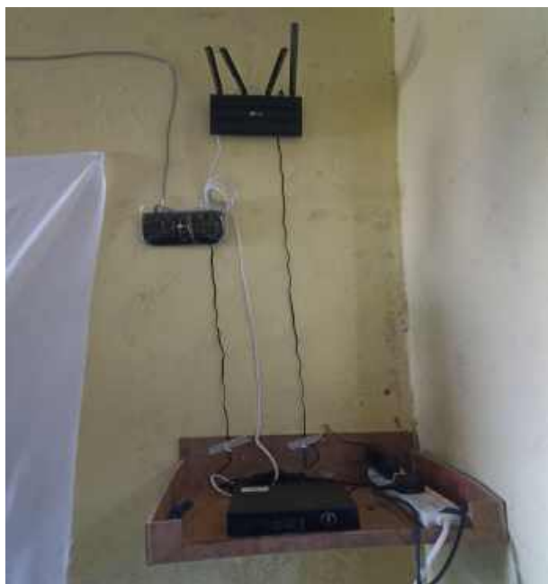
Offline server connected with router and switch
